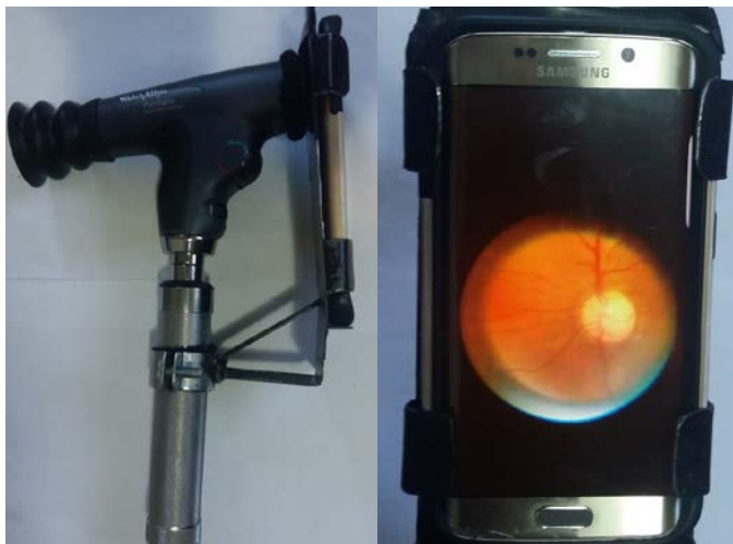
Figure 1: Welch Allyn Panophthalmoscope with Samsung Galaxy S6 Edge and one field of view
